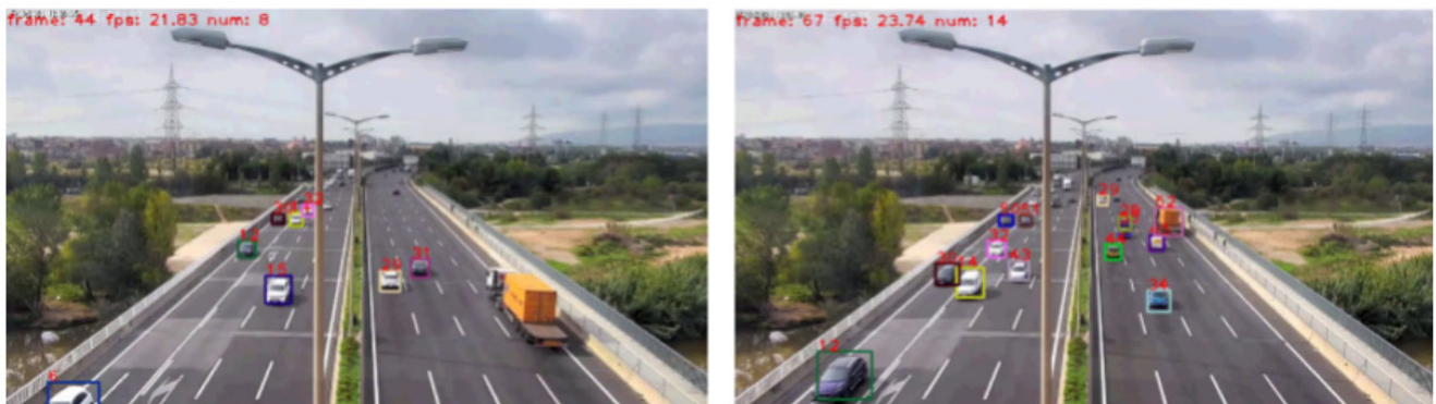
Figure 9: Detection and tracking with YOLOX and BoT-SORT in 2 frames separated by about 2 seconds in a highway setting.
