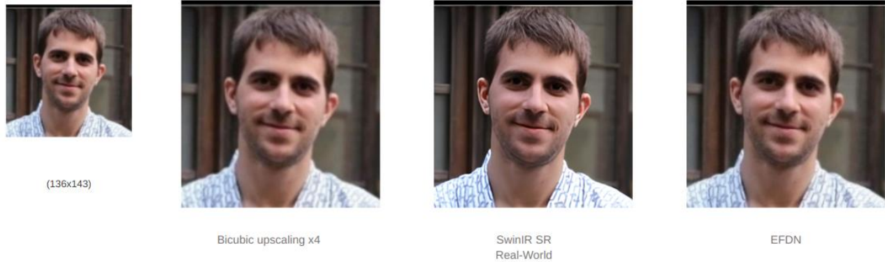
Figure 46: A qualitative comparison of different Super-Resolution (SR) algorithms on an image displaying a face.
