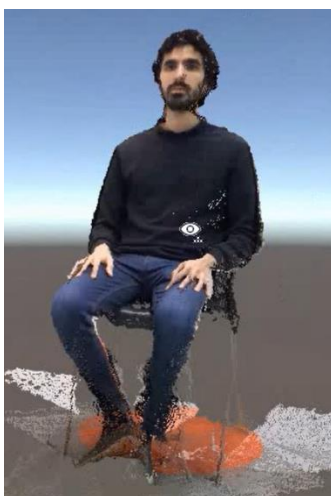
Figure 74: Real-time point cloud capture at 15 fps with 750K points per frame.
