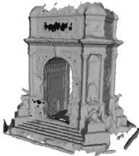
Figure 37: Result of a naïve mesh cleaning process run on a model of Arco Valentino.
