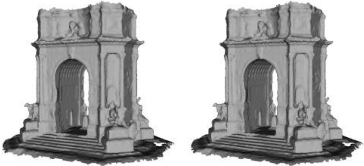
Figure 39: Two meshes representing Arco Valentino with ~200k (left) vs. ~20k (right) vertices.
