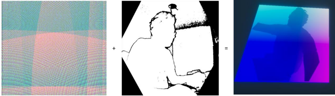
Figure 71: 2D to 3D RGB-D image mapping. From left to right: Intrinsics map, depth map, the resulting position map.
