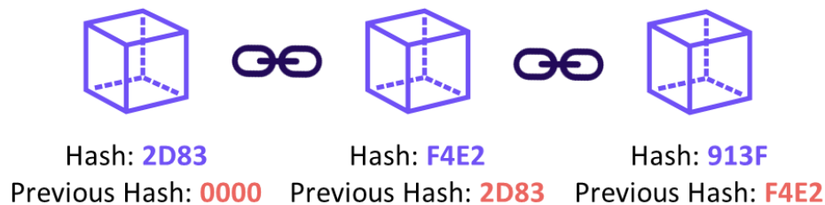
Figure 8-9 How blocks are chained.
