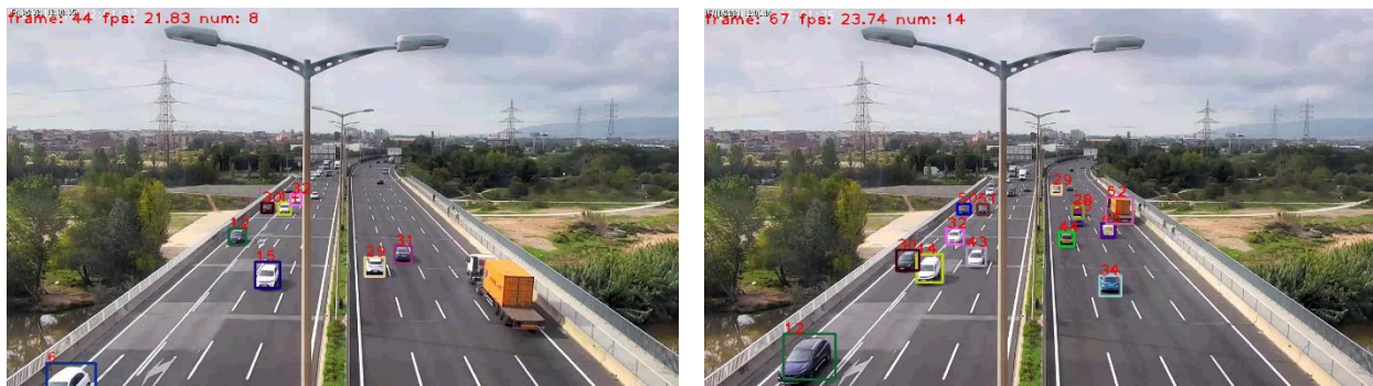
Figure 4-21 Detection and tracking with YoloX and BoT-SORT in 2 frames separated by about 2 seconds
